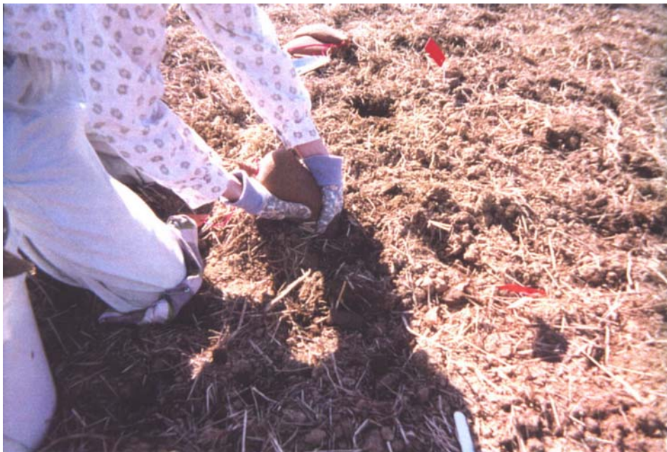
Figure 2b. Burying soil bags in cored holes.
