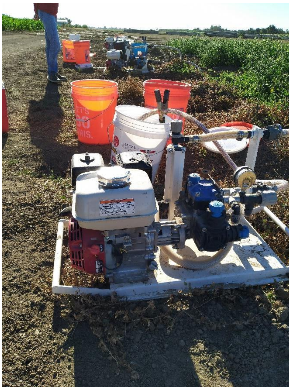
Figure 1. Fertigation system consisting of a pump and buckets filled with the amendments diluted in water. Photo taken June 8, 2020.
