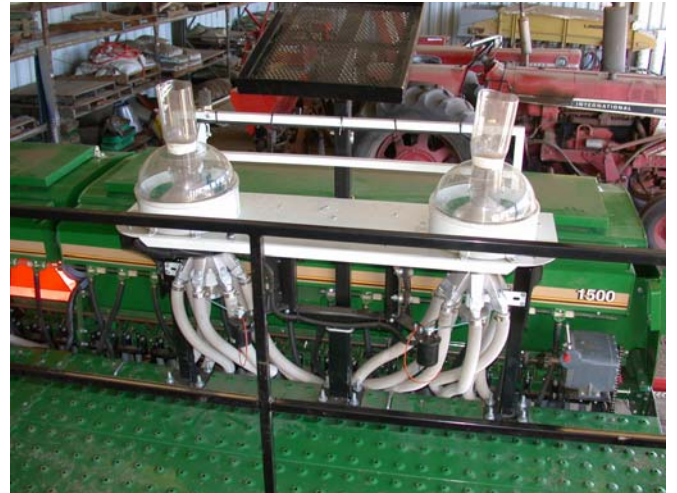
Photograph 2. Seed cones on research grain drill for precision planting.
