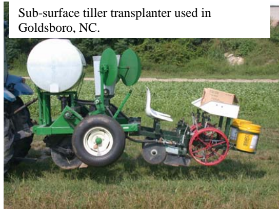
Transplanting operation in Goldsboro, NC: September 2, 2004. In areas of high residue, manual closure of the planting furrow was required around some plants.
