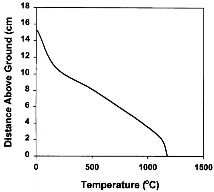
Fig. 2. Effect of distance from burner on the temperature experienced by the plant.
