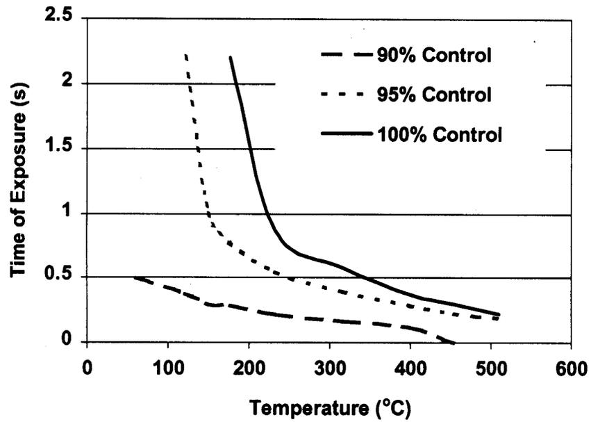
Fig. 1. Effect of temperature and time of exposure on the efficacy of flaming for killing plant tissue. Source Lalor and Buchele, 1968.
