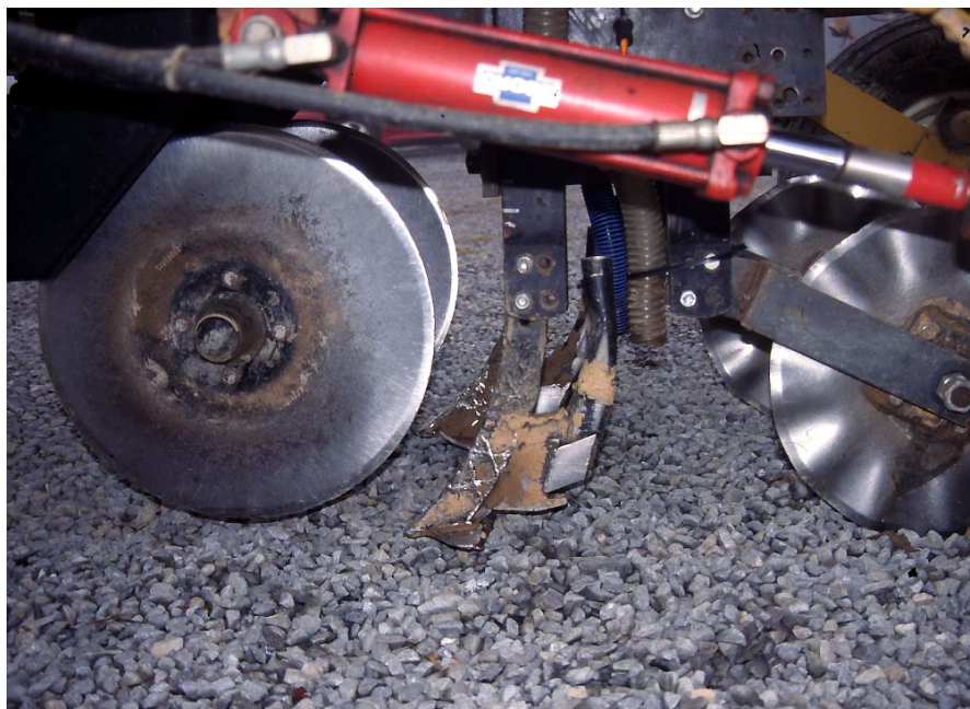
Figure 2. Upper (U)—SST-T planting potato seed pieces in living rye cover crop. Lower (L)—Underside view of SST, showing twin-row configuration (left to right), 20-inch straight counters to slice rye, wide-wing subsoil shanks to till (loosen) soil in potato grow zones and attached tubes to surface band organic fertilizer in grow zones, and 18-inch wavy coulters to incorporate the fertilizer in the grow zones. Two NT planters (not shown) were mounted directly behind the wavy coulters to set potato seed pieces 5-6 inches deep in the grow zones.
