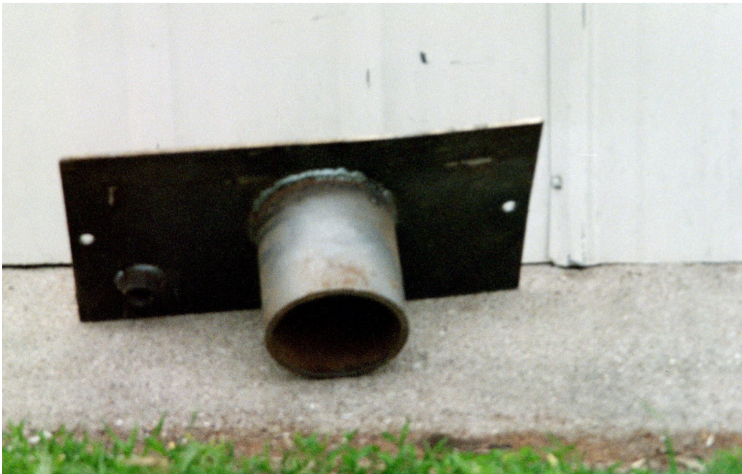
The attachment we mounted to the loader bucket, which enabled us to push the posts in the ground
